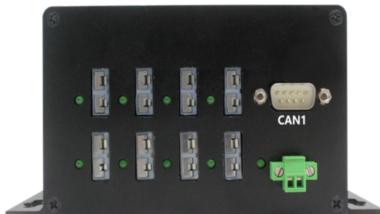
Figure 1-2 Hardware Interface (CAN FD)
